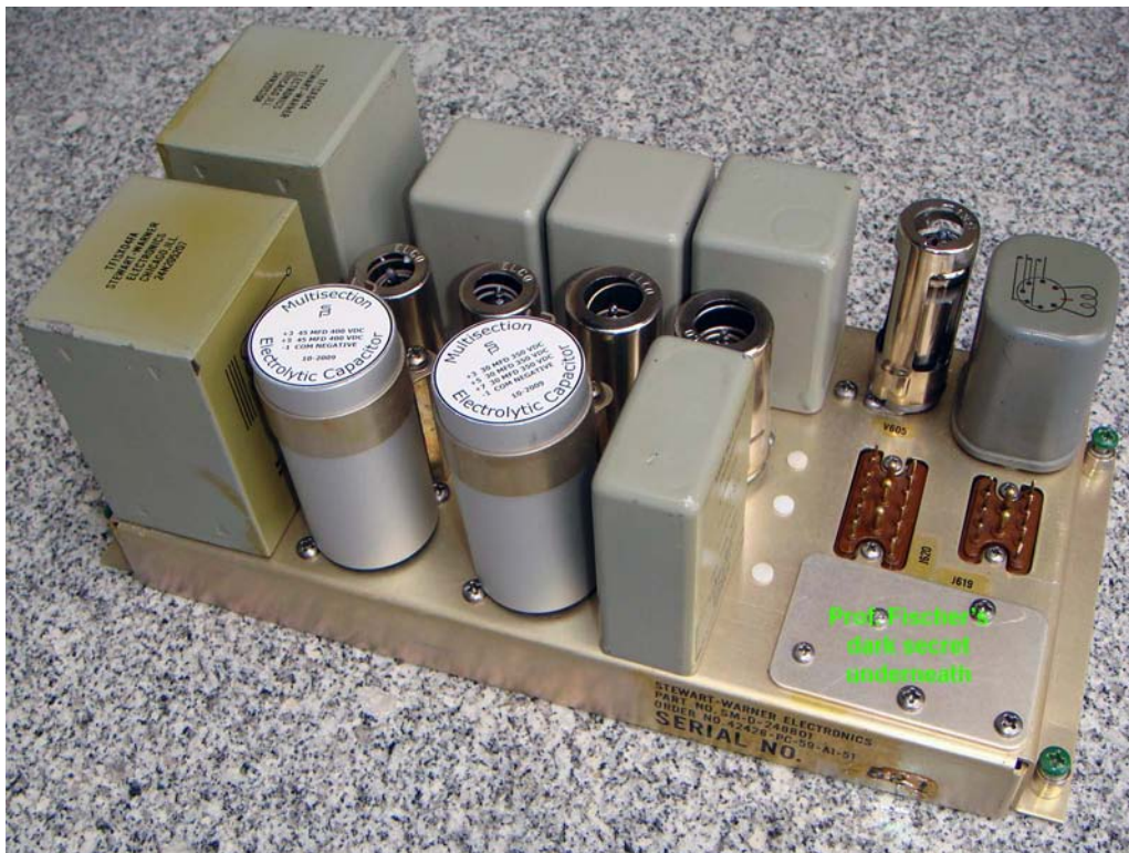
Fig. 3 Stewart-Warner audio module recapped with new electrolytic capacitors C603 & C606
