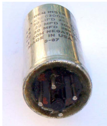
Fig. 1 Refilled multi-section electrolytic capacitor after 14 years of flawless operation in its 'new life'
