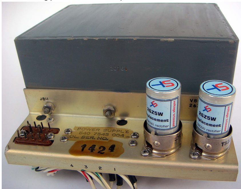
Fig. 2 Power supply chassis equipped with a pair of 26Z5W replacement modules (tube shields are no longer necessary)
